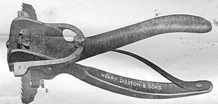
Specially adapted for Hand Saws, Cross-Cut Saws, Circular Saws, and all small saws.
